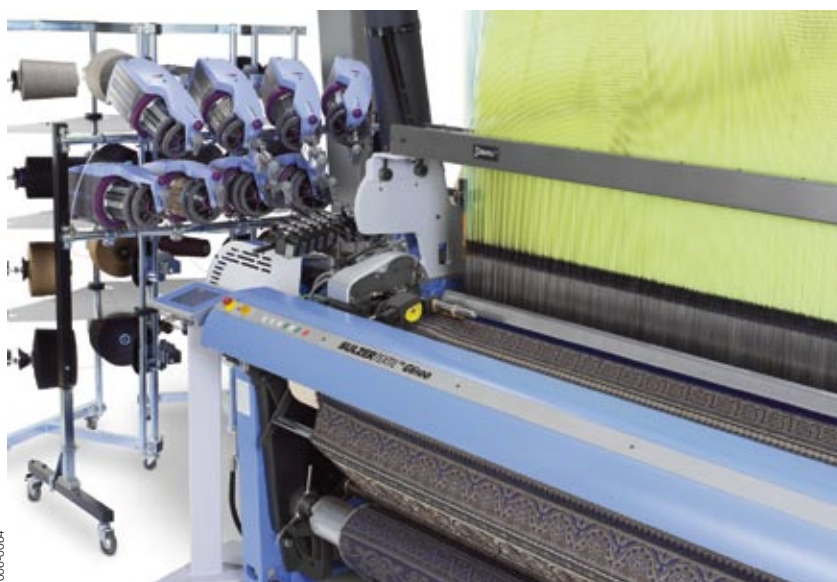
For curtain and furniture covering fabrics the G6500 can weave different weft yarns simultaneously, e.g. spun-fibre, coarse fancy, loop and bouclé yarns.
